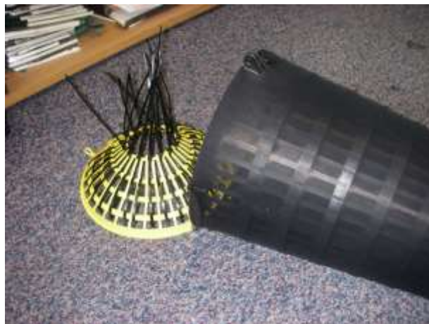
Figure 8. Deluxe trappy trap covered in stocking material, also the zip ties coming off from the funnel can be observed.
