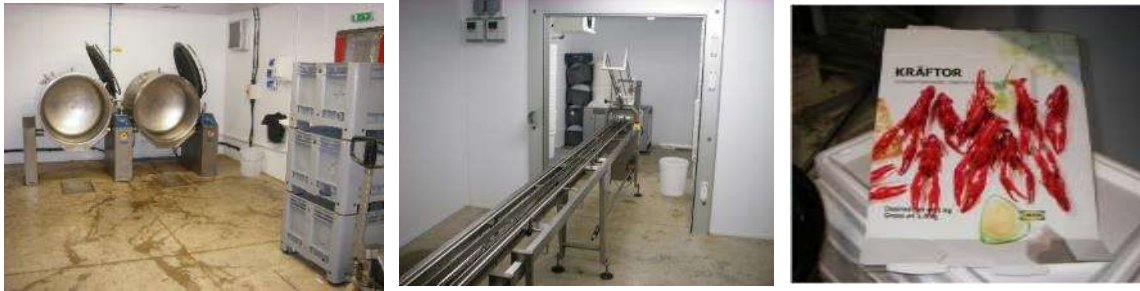
Figure 2. Images from the crayfish processing plant, showing the a) cooking and b) packing equipment, in addition to c) the packaging itself.
